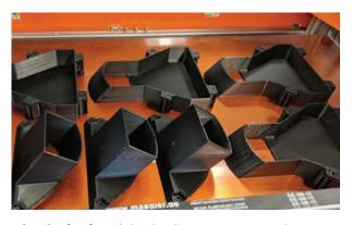
**Boyce Technologies** found that lead times on previously outsourced parts could be nearly eliminated by manufacturing parts in-house overnight using "lights off" additive manufacturing processes.
