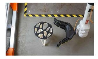
The Adaptive Robotic Gripper demonstrates the power and flexibility of BigRep's technology to create custom solutions for the factory of the future. Fully 3D printed and customizable for specific needs.
