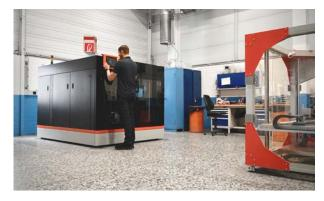
**Ford** invested in the BigRep PRO for faster speeds to meet their growing demand for additively manufactured tooling, like jigs and fixtures, and for engineering-grade materials to create end-use parts.
